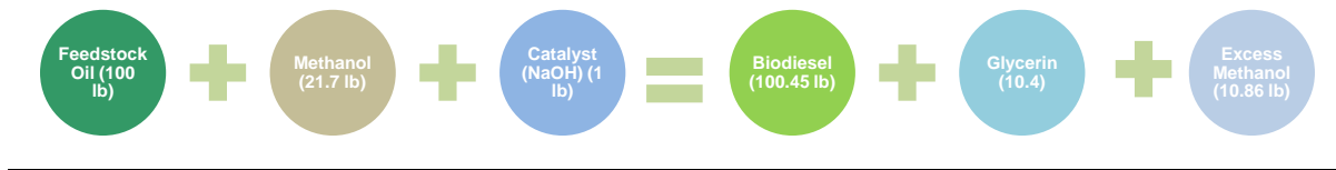
Figure 9: Biodiesel Production – Transesterification Process
